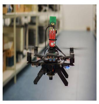
Imec IDLAB demo of high-accuracy UWB localization of drones in a warehouse
