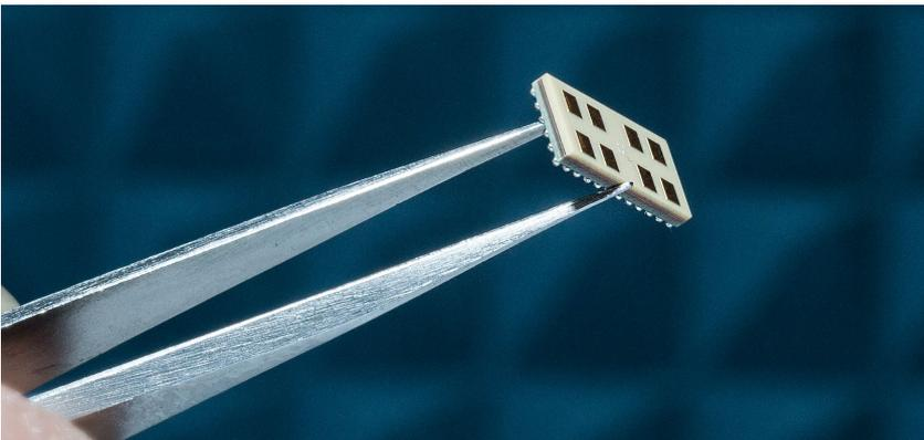
*Prototype of imec's multi-Gb/s 60GHz wireless transceiver*
