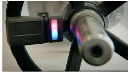
The Aloxy sensor is fitted to the operating hand wheel of manual valves and so is easy to implement.
