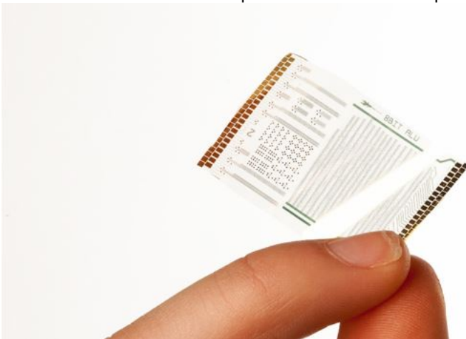
Thin film microprocessor on plastic film.
