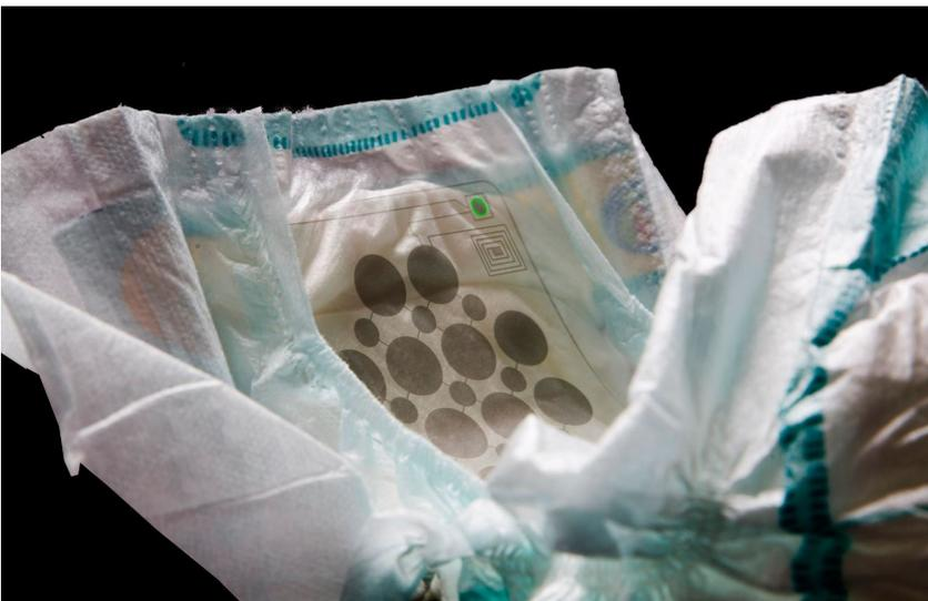
In the future, crèches are likely to use diapers fitted with a moisture sensor and (NFC) tag: all the carer has to do is place her smartphone close to the diaper and the tag will tell the smartphone whether the diaper is wet or not.
