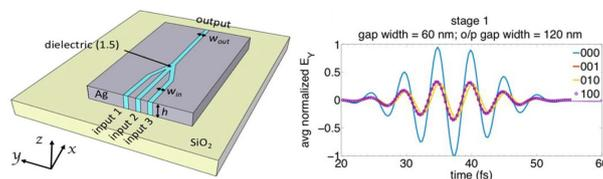
Plasmonic majority gate: (left) schematic representation and (right) output of a single stage majority logic gate displaying the results for the case of majority logic 0.
