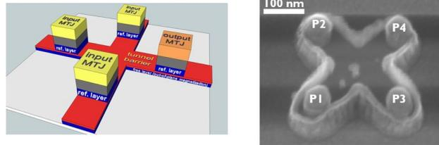
*Spin torque majority gate: (left) schematic representation and (right) integrated device.*
