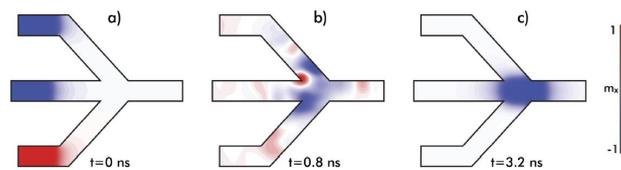
Simulation of the operation of a nanoscale spin-wave majority gate. (a) At  $t=0\text{ns}$ , the inputs are set to '110'; (b) at  $t=0.8\text{ns}$ ; and (c) at  $t=3.2\text{ns}$ , the output magnetization is stabilized to the '1' state, correctly detecting the majority result. Total area of the device is about  $0.05 \mu\text{m}^2$ .
