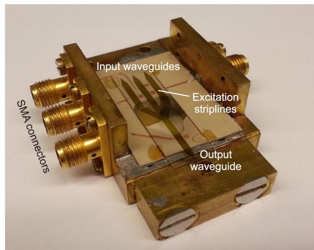
*Large-scale prototype of a spin-wave majority gate.*
