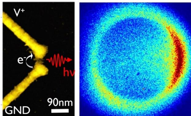
*(Left) Imec's ultra-small antenna-coupled tunnel junction demonstrating unidirectional light emission (right).*
