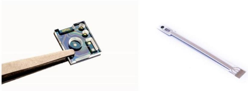
*There are two versions of the fluid sensor: one on silicon and the other on a bendable substrate.*
