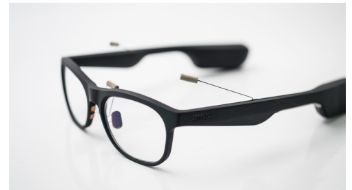
imec's newest prototype with enhanced EOG performance and an optimized, ergonomic design
