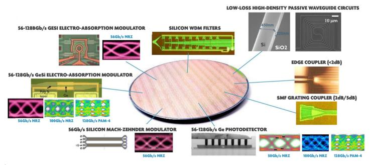
Imec's versatile 50G+ silicon photonics platform
