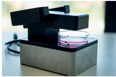
Detailed view of acquisition stage of the lens-free microscopy evaluation system
