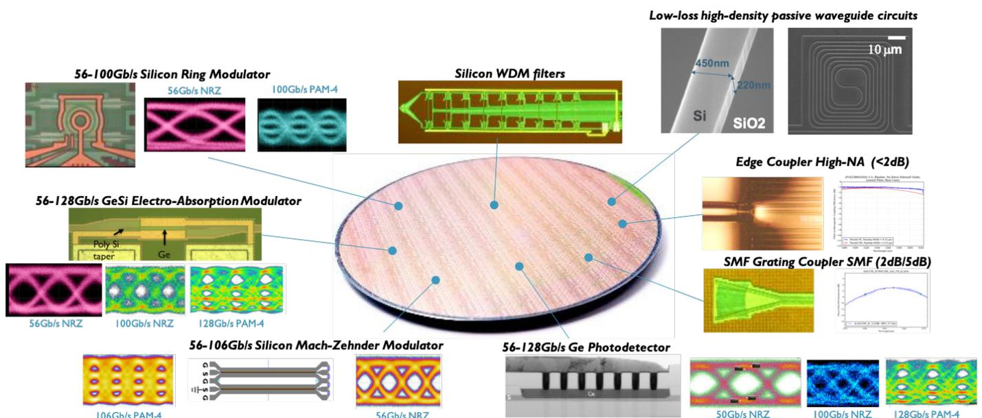
Imec's versatile 50G+ silicon photonics platform
