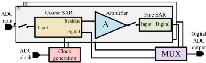
Figure 4: Architecture of the ADC
