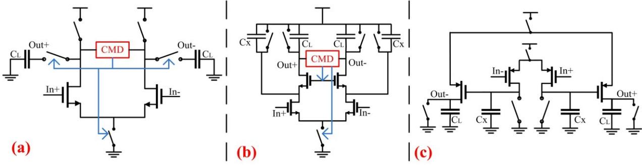
Figure 1: Schematics of different dynamic amplifiers
