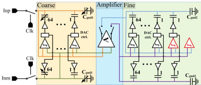
Figure 5: Detailed implementation of the ADC
