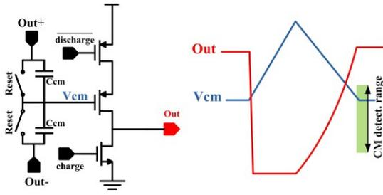
Figure 3: the CMD and its waveforms
