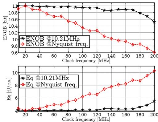
Figure 10: ENOB and FoM of the ADC @ 10 MHz input and Nyquist
