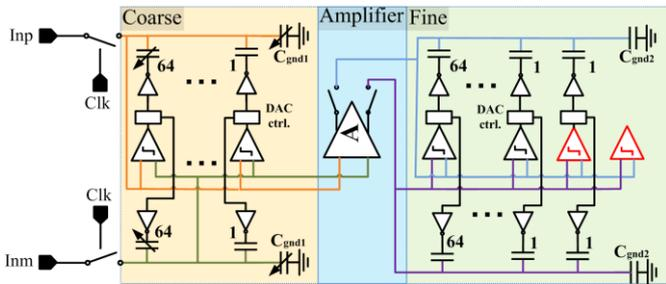
Figure 5: Detailed implementation of the ADC
