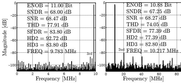
Figure 8: FFT @ 20 MS/s and 170 MS/s
