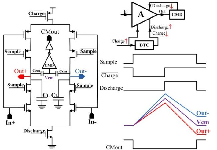
Figure 2: Complementary dynamic amplifier and its waveforms
