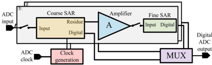
Figure 4: Architecture of the ADC
