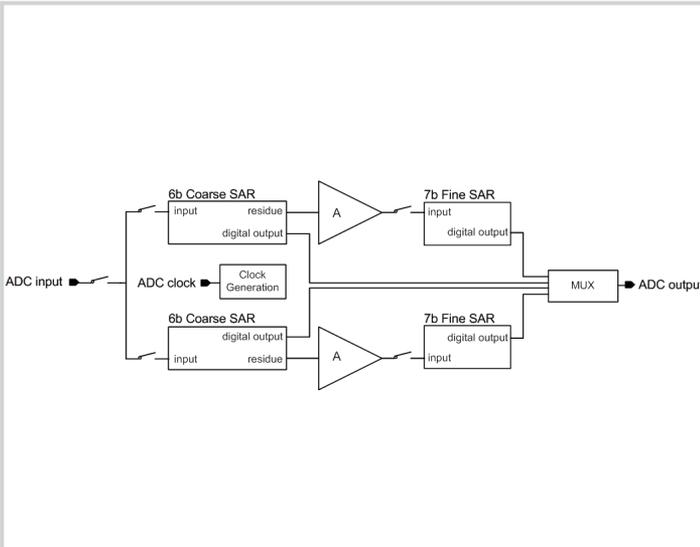
Figure 27.5.1: Block diagram of the implemented ADC.
