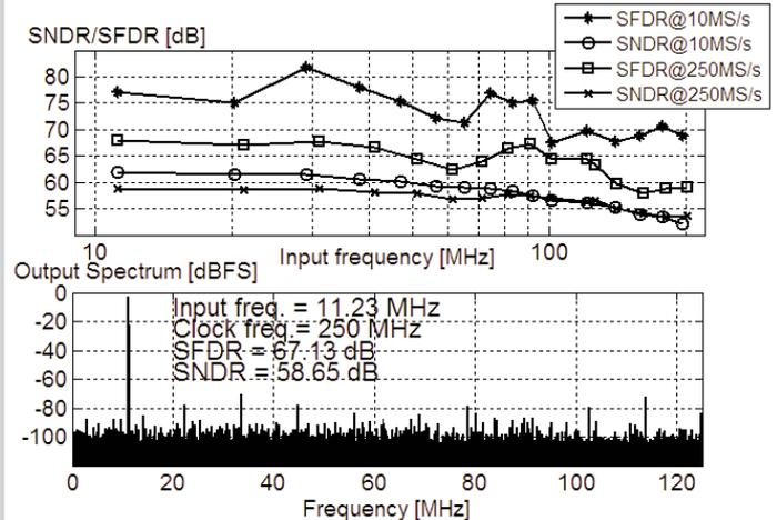
Figure 27.5.5: SNDR/SFDR vs. input frequency at 10MS/s and 250MS/s sampling frequency (top) and measured output spectrum at 250MS/s (bottom).
