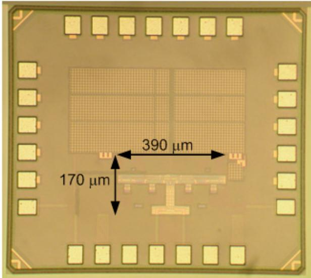
Figure 27.5.7: Chip micrograph with core size indicated.
