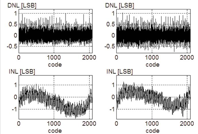
Figure 27.5.4: DNL (top) and INL (bottom) of channel 1 (left) and channel 2 (right) of the ADC.
