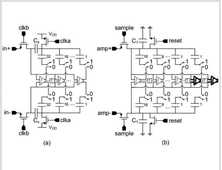
Figure 27.5.2: Simplified architecture of the coarse SAR stage (a) and the fine SAR stage (b).
