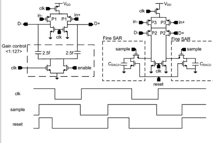
Figure 27.5.3: Schematic of the dynamic residue amplifier and clock waveforms for this amplifier and the fine SAR.
