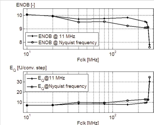
Figure 27.5.6: Measured SNDR and SFDR (top) and energy per conversion step (bottom) as a function of clock frequency.
