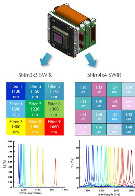
Snapshot mosaic hyperspectral image sensors with  $3 \times 3 = 9$  colors and  $4 \times 4 = 16$  spectral bands. Each filter is patterned at pixel level and integrated into the Cardinal 640 InGaAs image sensor from SCD
