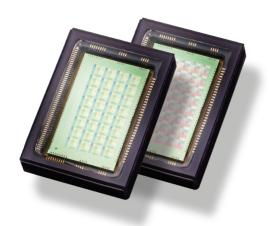
Packaged hyperspectral snapshot mosaic, 16 and 25 bands, hyperspectral image sensor from imec
