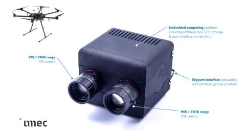
UAV purpose multi-camera hyperspectral Imaging system carrying two hyperspectral imaging cameras (VIS to SWIR range) with embedded computing platform and Skyport connectivity for seamless acquisition and processing of hyperspectral imaging data in real-time.
