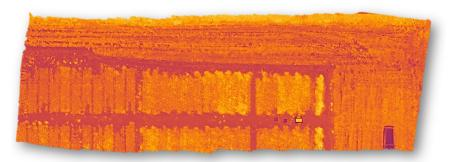
NDVI (vegetation vigor index) orthophoto stitched images acquired from several test flights data by imec team in Belgium. The full HW & SW pipeline platform has been early on validated in order to ease the integration and deployment of this unique technology in low altitude drone projects.
