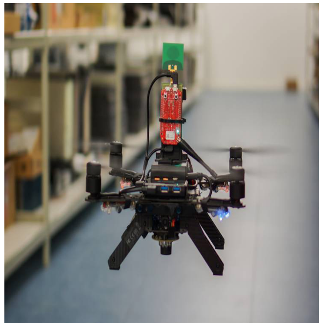
Imec IDLAB demo of high-accuracy UWB localization of drones in a warehouse
