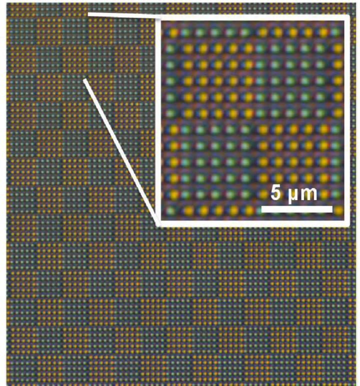
RGB camera measurement (100x magnification) of an array of waveguides with alternating 5 left-side-open-aperture and 5 right-side open-aperture (the others being occluded by TIN) waveguides at a 1-micron pitch. Yellow light exits at the right part of the waveguide, whereas the blue exits at the left. The wafer is illuminated using plane wave white light.
