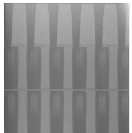
3D visualization (left) and TEM cross-section (right) of the vertical waveguide array for color splitting in BY-CR imaging.
