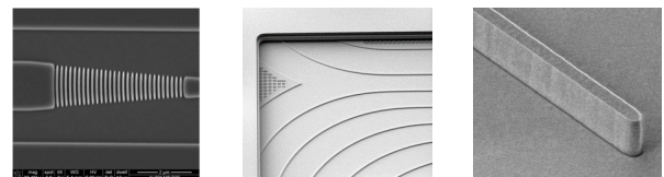
Examples of fine patterning of optical components e.g. grating, waveguides and taper
