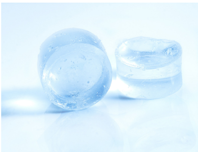
Solid electrolyte monolith pellets casted in a mold from imec's patented nanoporous SCE material liquid precursor
