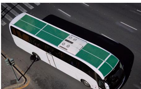
Application for thin-film solar cells
