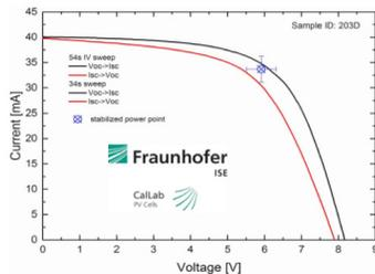
Certified efficiency of 12.4% for perovskite module with 16cm<sup>2</sup>
