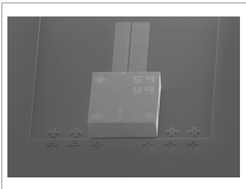
Scanning electron-microscope image of an InP DFB laser assembled on a Si Photonics chip
