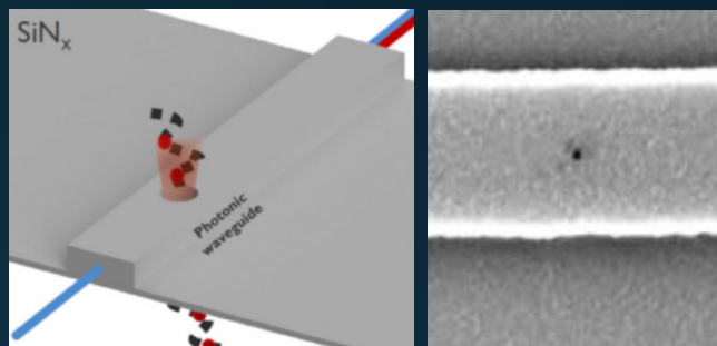
Illustration and SEM image of an integrated photonic nanopore device for fast, scalable single-molecule fluorescence-based detection.
