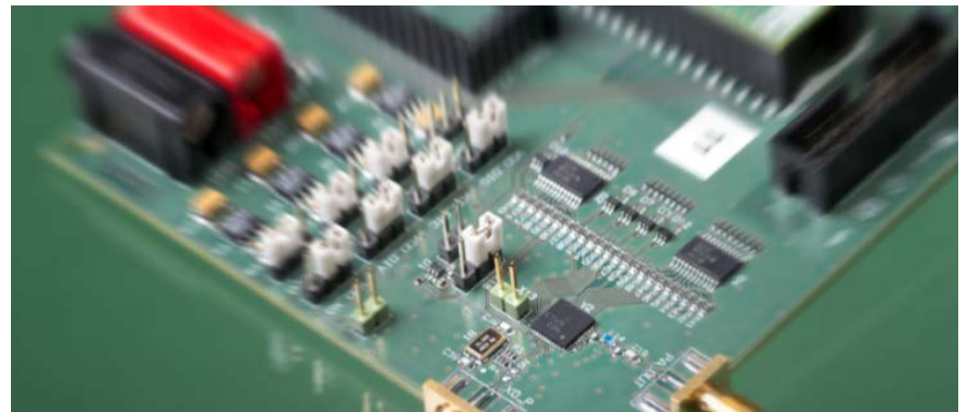
Evaluation PCB: Allows complete evaluation of the 2.4 GHz All-Digital PLL.
