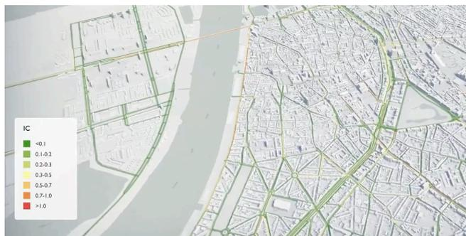
Figure 2: User interface of the first Urban Digital Twin created for Antwerp in 2018.
