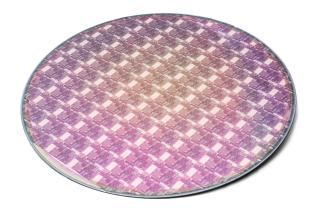
A 300mm wafer processed on imec's iSiPP platform
