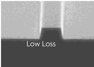
Left: Extremely low loss SiN rib waveguide Right: High quality factor SiN ring resonator; (LPCVD)
